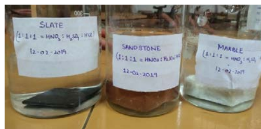
Figure 7: Stones dipped in equinormal solution of acids (1:1:1 of H 2 SO 4 : HNO 3 : HCl).
