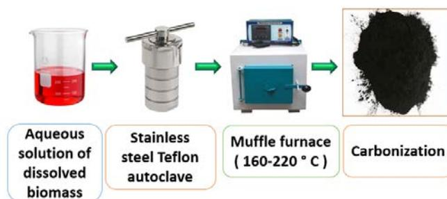
**Figure 6:** Schematic diagram of hydrothermal synthesis of mesoporous carbon.
