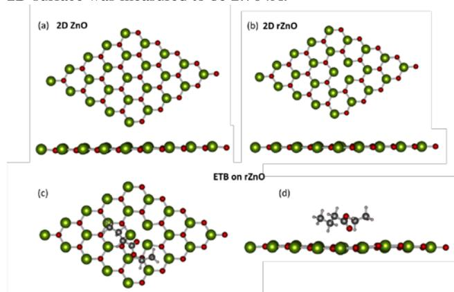
**Figure 1:** Supercell of (a) 2D ZnO and (b) 2D reduced ZnO (rZnO), showing views from the top (XY plane) and side (YZ plane) (c) top view of ETB molecule adsorbed on rZnO and (d) side view of ETB molecule adsorbed on rZnO.
