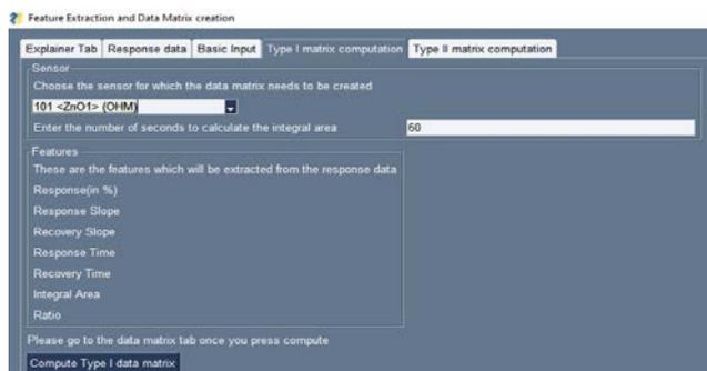
Figure 8 (a) Screenshot of computation of a type I data matrix with all the features of a particular sensor
