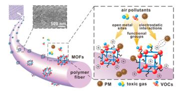
**Figure 6** Representation of MOF-based polymer and filtration of air pollutants. Reprinted with permission from Ref. [73]. Copyright 2016 the American Chemical Society.
