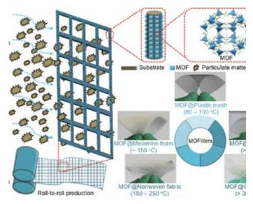
**Figure 7**. Representation of filtration materials prepared using MOF with roll-to-roll hot-pressing strategy. Reprinted with permission from Ref. [69]. Copyright 2017, WILEY-VCH.
