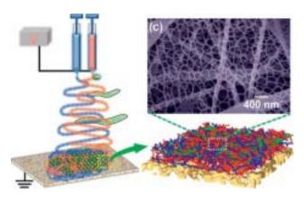
**Figure 3.** Electrospinning technology for nylon-6/PAN nanofiber/net membranes creation. Reprinted with permission from Ref. [60], copyright 2015, The Royal Society of Chemistry.
