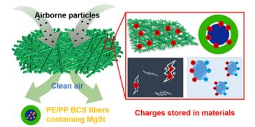
**Figure 4.** Magnesium stearate as charge enhancer in PE/PP nanofiber based electret filter. Reprinted with permission from Ref. [61], copyright 2019, American Chemical Society.
