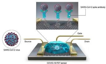
**Figure 9.** Representation of Spike antibody immobilized graphene for FET sensor for Covid-19 diagnosis. Reproduced from [141] with unrestricted reuse permission by ACS for Covid-19 work. Copyright © 2020, American Chemical Society.
