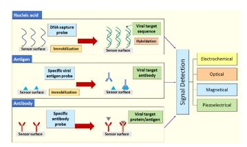
**Figure 8.** Summary of different methods and signal detection in biosensors meant for SARS and MERS coronaviruses. Reproduced from ref [122] Creative commons license CC 4 By.
