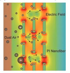
**Figure 5**. Image depicting the filtration process through R-TENG filter. Ref. [65], copyright 2017, American Chemical Society.
