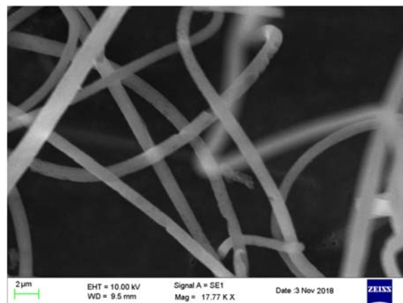
Figure 1(c): SEM micrograph of 10 wt % CNF
