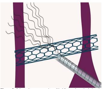
**Figure 3.** Schematic representation of holding and manipulating the nanoscale materials in a nano optical tweezers. "Acknowledged [biorender.com] as per instructions".
