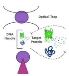
three-dimensional with high-resolution by forwarding scattered light. Optical tweezers are used to grab single molecules and measure events that are occurring and employed for measuring forces and measuring distances. A miniature and modular system creates a reliable and mobile optical trap that has more potential to be applied in optical trapping technologies.
