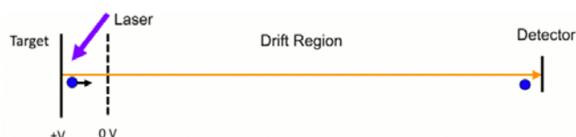
Figure 4: Schematic description of TOF-MS process; Taken from 15 , licensed under CC-BY-SA 4.0.
