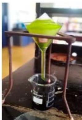
Figure 3: Filtering the solution after 48hrs.
