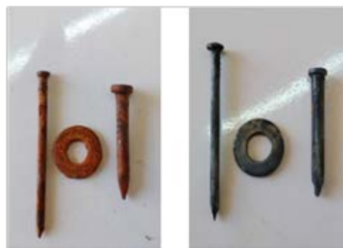
Figure 29. (A) Without wax (B) With wax coated
