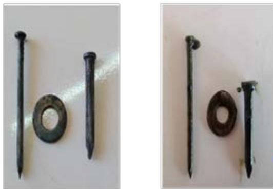
Figure 26. (A) Without coating of wax. (B). With wax coated
