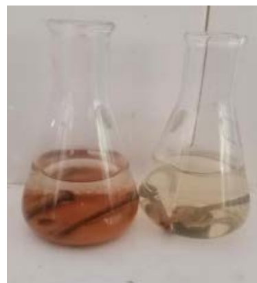
Figure 28: After a month of dipped iron materials in water.
