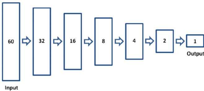
Figure 3. Number of layers used in the multilayer perceptron for image compression
