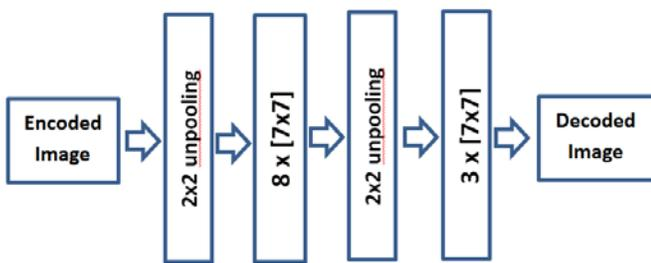
Figure 11. Decoder network for CNN-AE-FT. Encoder part is same with CNN-AE
