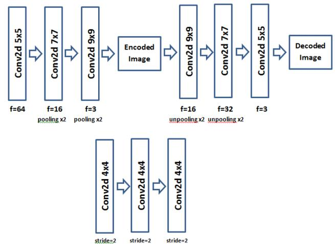
Figure 9. Generator of GANs being using as a decoder
