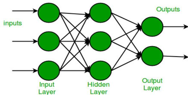
**Figure 12.** Architecture of multilayer perceptron network
