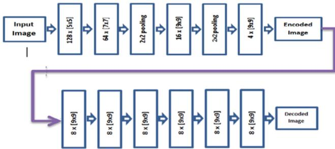
Figure 6. Convolutional autoencoder for encoding and decoding of image.
