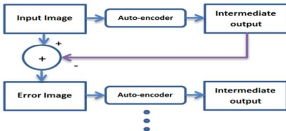
Figure 7. Recurrent CNN-AE for introducing a trade-off between image quality and compression ratio.
