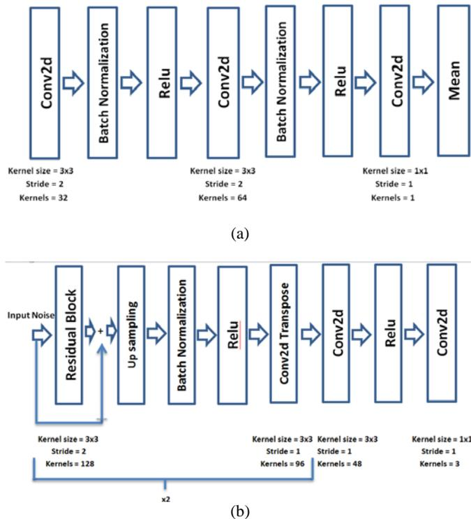
Figure 10. Compression achieved using combination of both auto encoder (a) and GAN (b)
