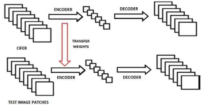
Figure 8. Fine-Tuning approach used for images specific compression
