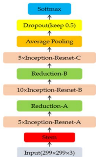
Figure 2. The construction of Inception-ResnetV2.
