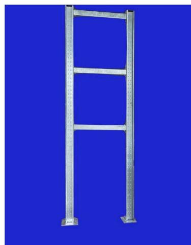
**Figure 2** Built-up cold-formed steel frame -Experiment model
