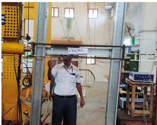
**Figure 16** observation and Recording of local buckling failure at the end of test
