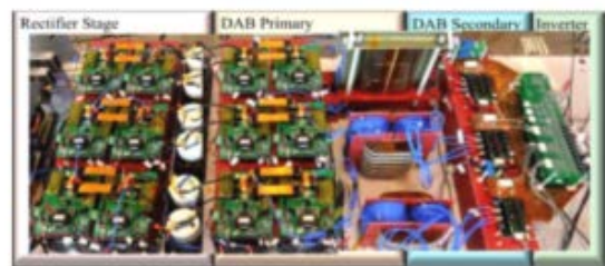
Figure 1. The external appearance of the high-frequency solid-state transformer.
