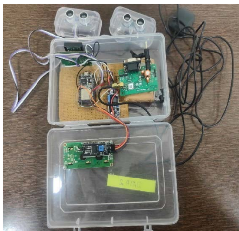
Figure 3: The Smart Waste Management Kit provided to Home Users
