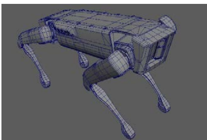
Figure 4a. Virtual model of Quadruped robot
