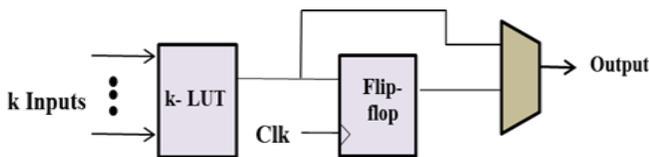
Figure 1: General Basic logic element (BLE) structure.
