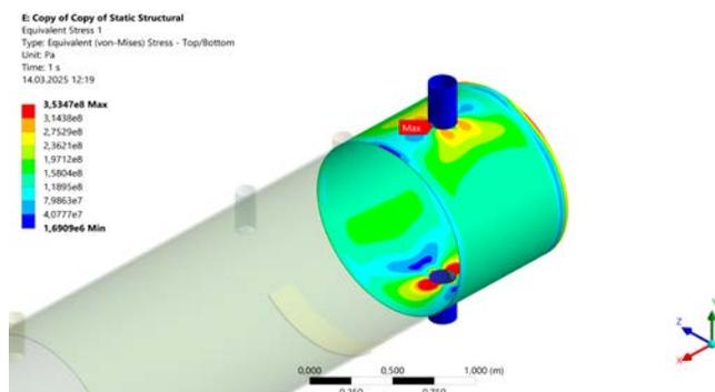
Figure 12. Stress in the first section with a nozzle A1 thickness of 6 mm
