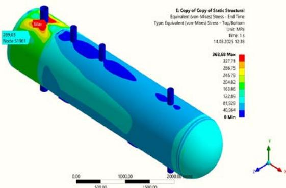
Figure 9. Vessel finite element model
