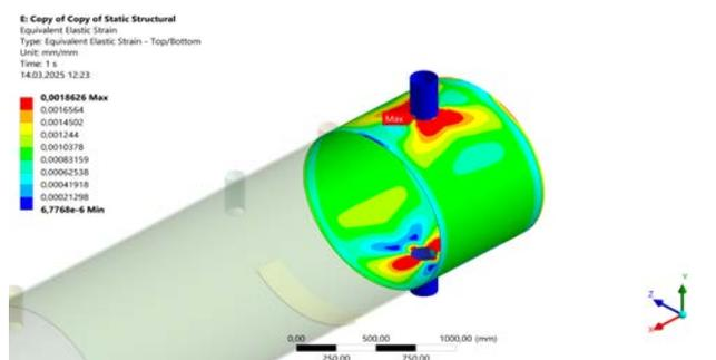
Figure 14. Residual plastic deformations
