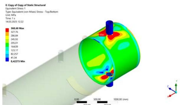
Figure 13. Stresses in the first section with a nozzle A2 thickness  $t \approx 5.6$  mm
