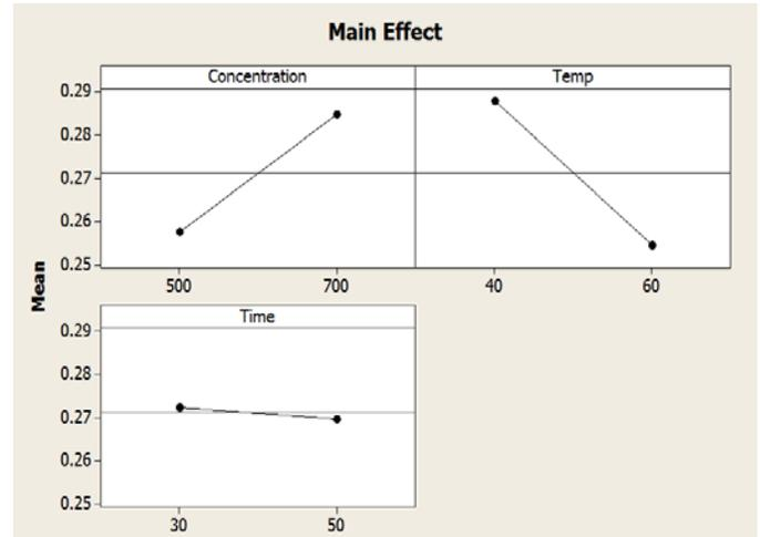
Figure 4 Effects of Concentration, Temperature, and Time on Etching Depth
