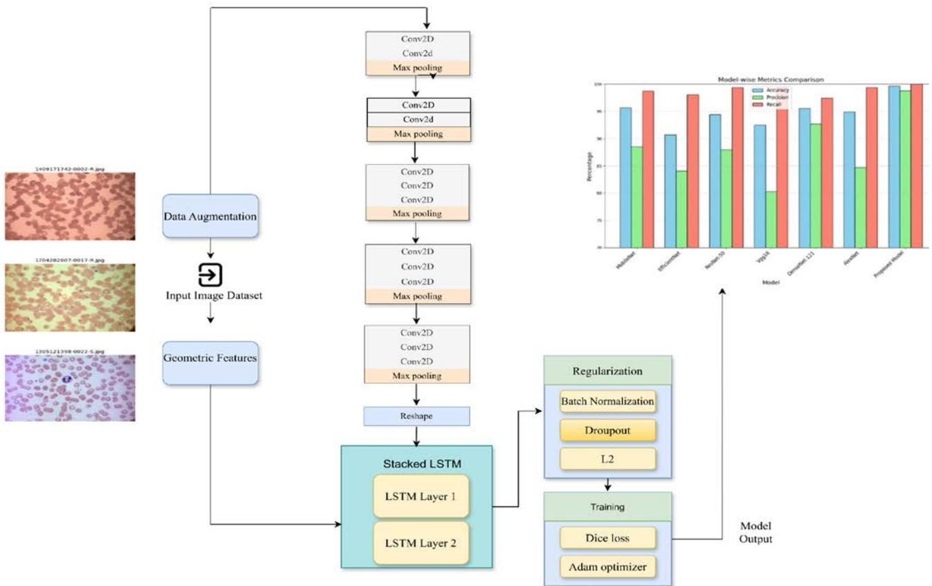
Figure 3. V2SeqNet - VGG with 2 LSTM Layers for Sequential Classification Network
