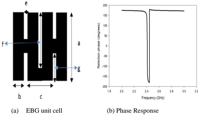
Figure 4. EBG a) Proposed EBG unit cell b) Its Phase Response
