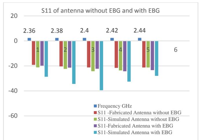
Figure 6 comparison of simulated and measured result of antenna without EBG and with EBG
