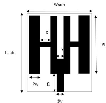
(a) Top View of Dual H shape antenna
