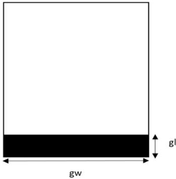
(c) Bottom View of Dual H shape antenna
