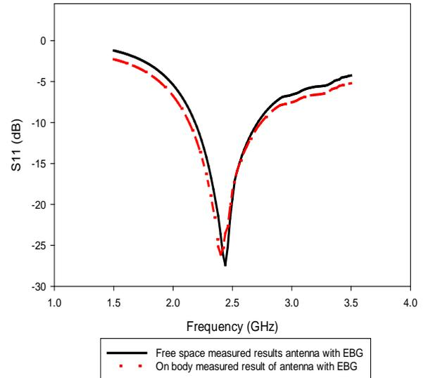
**Figure 11.**  $S_{11}$  of antenna with EBG in free space and on body
