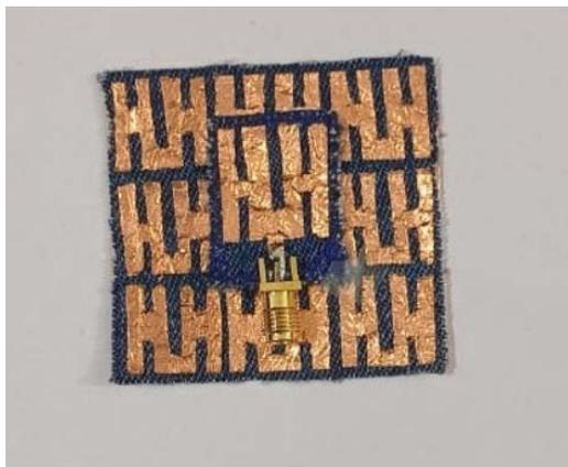
(a) Antenna incorporated with EBG array
