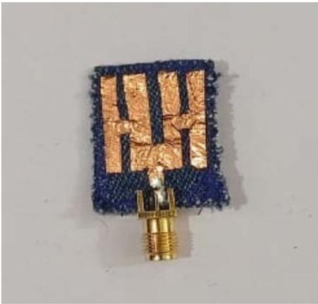
(b) Top View of fabricated Dual H shape antenna
