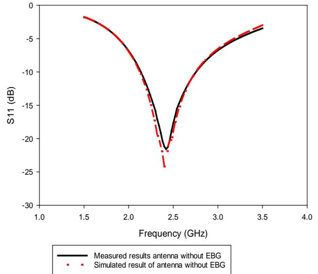
**Figure 2.** Comparison of measured and simulated reflection coefficient  $S_{11}$  of proposed antenna
