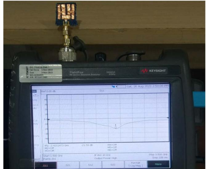
**Figure 3.** Fabricated antenna measurement on VNA
