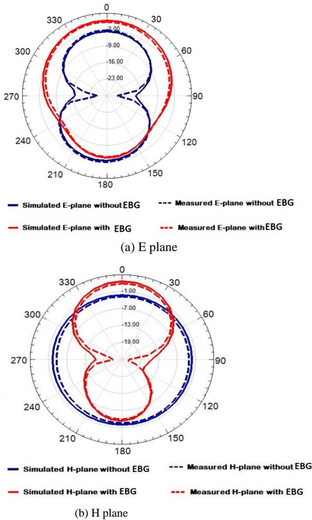
**Figure 7.** (a) Simulated and measured radiation patterns of antenna with EBG in (a) E plane and (b) H plane.
