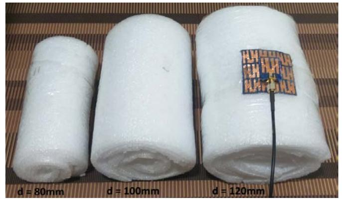
**Figure 8.** Fabricated foam cylinders with varying diameters
