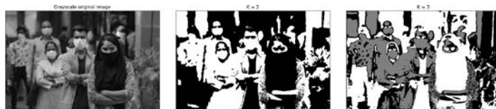
Figure 5. Detecting K-Means Clusters (From left a. original image, b. K=2, c. K=3)
