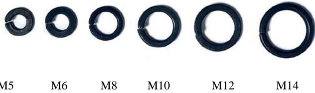
Figure 4: Image of washer samples
