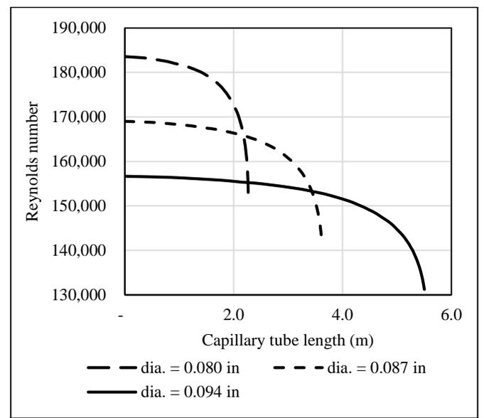
**Figure 9** The relationship between the Reynolds number and the length of the capillary tube
