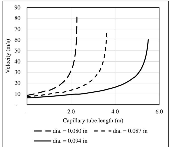
**Figure 8.** The relationship between the velocity and the length of the capillary tube
