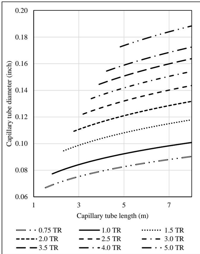
**Figure 14.** The optimum size (diameter and length) of capillary tubes for various cooling capacity
