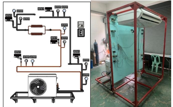
Figure 5 Experimental setup and instrumentation
