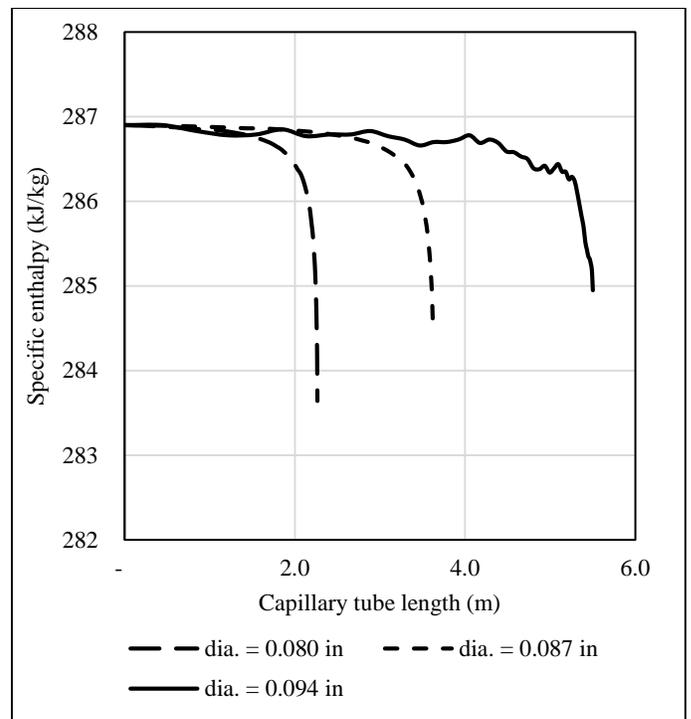
**Figure 12.** The relationship between the specific enthalpy and the length of the capillary tube
