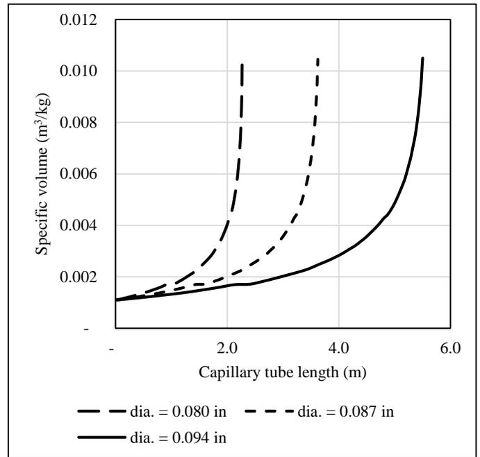
**Figure 11.** The relationship between the specific volume and the length of the capillary tube
