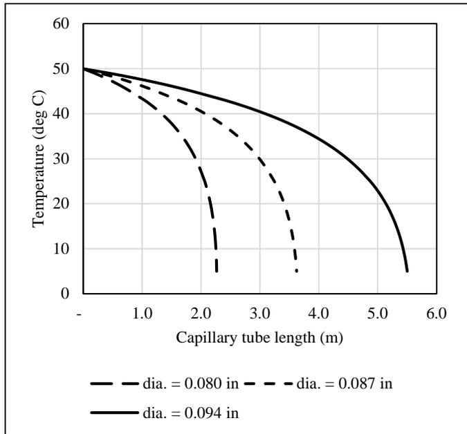
**Figure 6.** The relationship between the temperature and the length of the capillary tube
