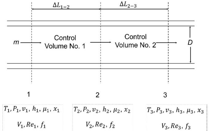
**Figure 1.** The schematic diagram for control volume in the analysis
