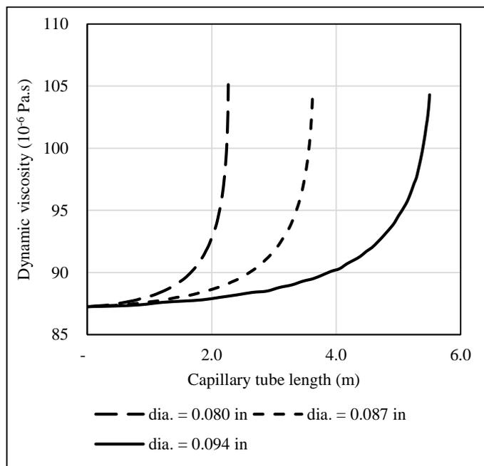
**Figure 13.** The relationship between the dynamic viscosity and the length of the capillary tube
