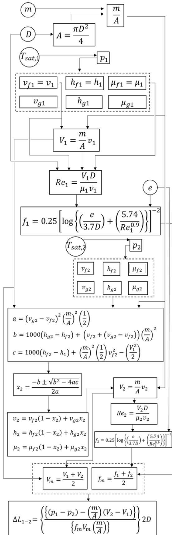
Figure 2. The analysis of capillary tube length of control volume 1, the primary parameters are in circles.
