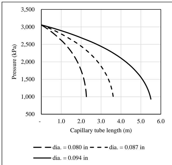
**Figure 7.** The relationship between the pressure and the length of the capillary tube
