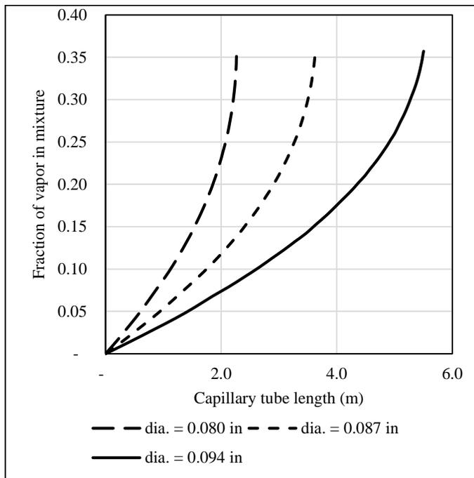
**Figure 10.** The relationship between the fraction of vapor and the length of the capillary tube
