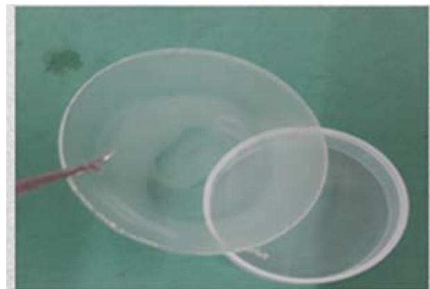
Figure 2. PMMA membrane (5% by PMMA+PVP wt.)
